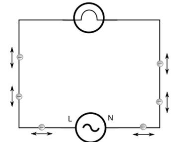
Negative current just means that the electrons are flowing in the opposite direction. Thus, instead of flowing from one place to another like in DC, the electrons just “rock” back and forth in the circuit.
