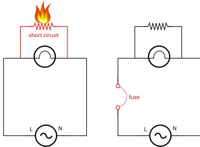
To prevent this, one uses either a **fuse** or a **circuit breaker**. Both of them are essentially switches that break the circuit once the current through it becomes too large, usually 10 A, 15 A or 20 A. A fuse needs to be replaced once it fires, while a circuit breaker can be reset.
