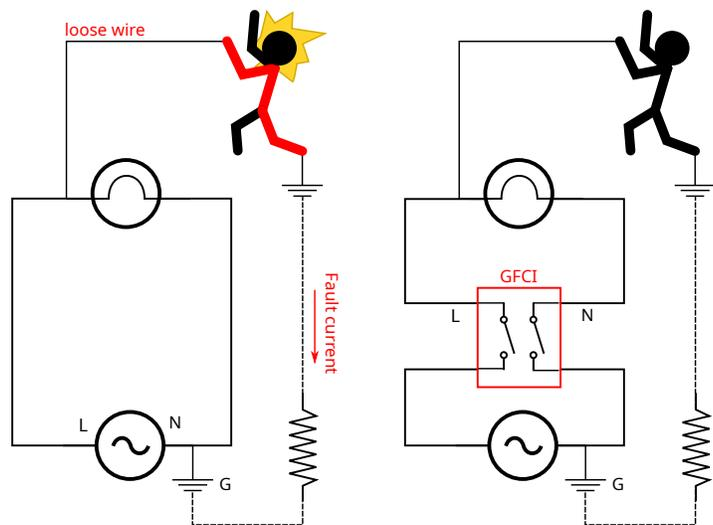
GFCI switches **rely on a good ground connection** (third pin in your plug) to detect fault currents, otherwise the resistance through the ground may be too large. This is why it is important to connect all your equipment to the ground to shorten the distance between the next good ground connection.
