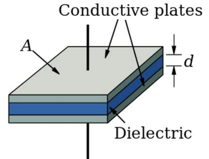
Because there is a “gap” between the two plates, it is important to note that **no electrons can move from one plate to the other**.
