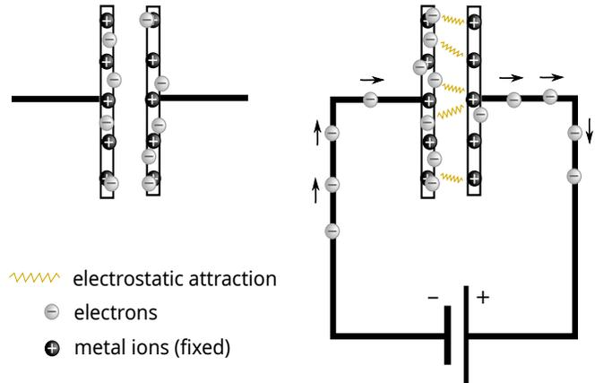
However, electrons repel each other, so the electrons should be pushed right back into the battery, right? No, some of the electrons can stay on the left side of capacitor since they are held in place by the attraction to the “+” ions on the right of the capacitor.
