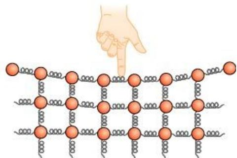
called **stress**. This is nothing but Hooke's law, which you found in the springs lab. A similar thing happens when **compressing** the material (the spring constant might be different). One can thus say that a spring behaves like a spring because it's made up of tiny springs (it's like *Inception* all over again).
